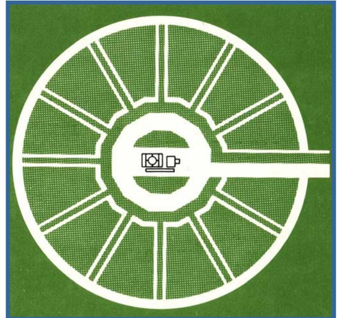
The time taken to reach this optimum size can be reduced by increasing the solids concentration present during flocculation. This is achieved in the Accentrifloc clarifier by recirculation of preformed floc.
